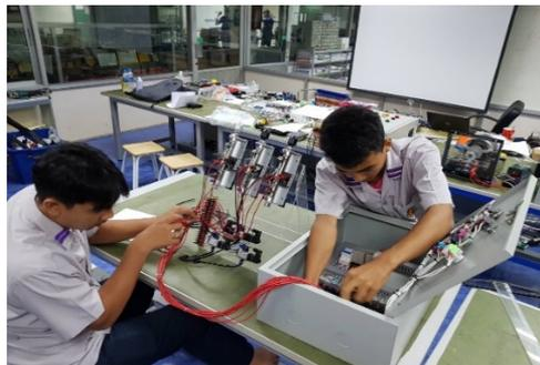
Figure 4. Pneumatic control project with relay circuit.
