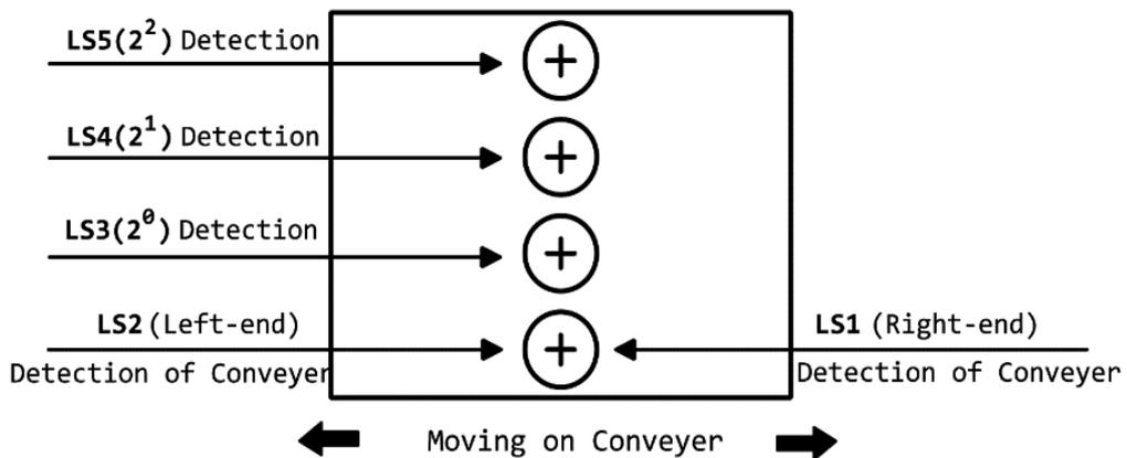
Figure 4. A pallet for sensing limit switch.
