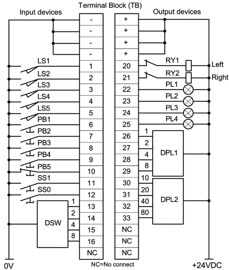
Figure 3. The Input and output devices diagram.
