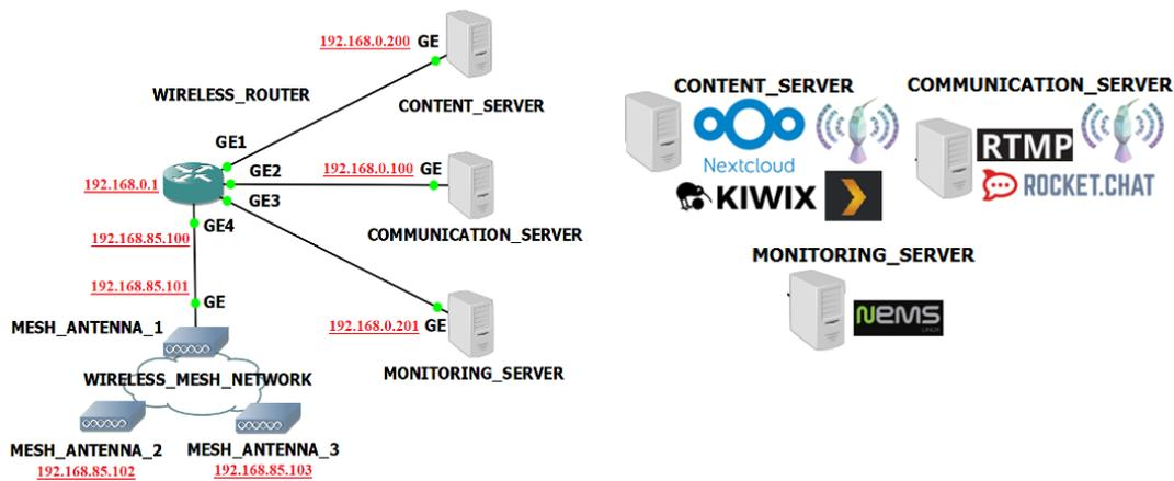
Figure 1. Mobile Network Diagram and Server Design.
