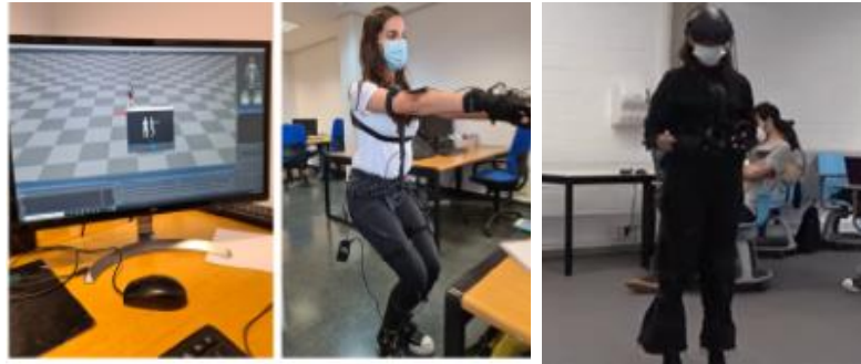
Figure 1. Perception Neuron Suit Calibration using Axis Neuron & Short Video Demonstration. https://youtu.be/r98GoEqEed0 .
